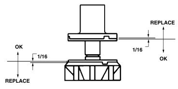
FIGURE 5. UPPER NUT AND BEARING ASSEMBLY
